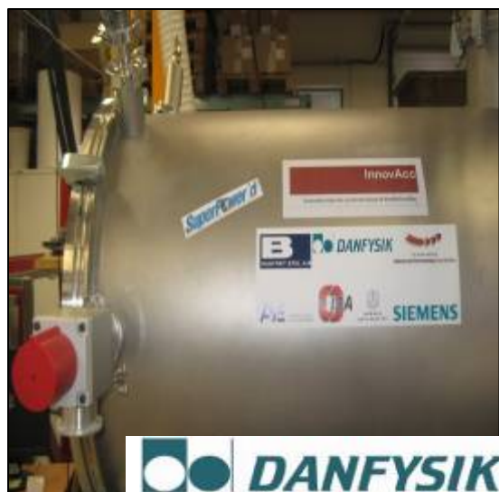
3.6 T gantry magnet for Particle Beam Therapy . Four racetrack coils and 14 bent coils. 2,500 m with min I_c of 115 A/4 mm.
