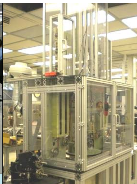
2011: I_c , n-value, thickness, width measurement in 10 m intervals
