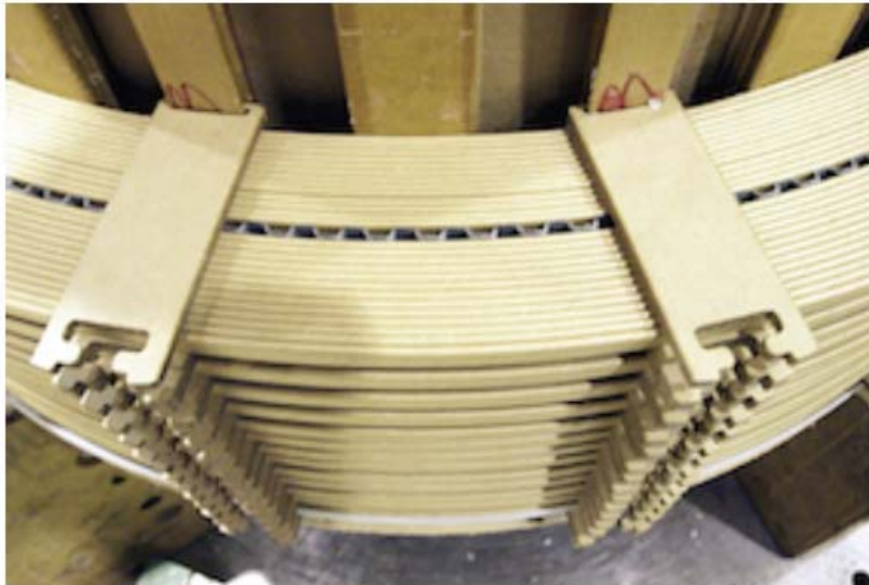
Example of Transformer Windings.
