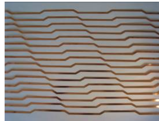
ROEBEL Cable Demonstrated by Karlsruhe Institute of Technology (KIT) with SuperPower ® 2G HTS Wire
