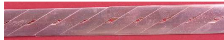
ROEBEL Cable Demonstrated by Karlsruhe Institute of Technology (KIT) with SuperPower ® 2G HTS Wire
