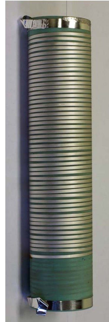
14.5 m of striated wire on a mandrel
